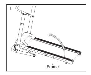
2. Pull the latch knob to the left and hold it. Raise the frame until the latch knob aligns with the hole in the frame guide, and release the latch knob. Make sure that the latch knob pin is fully inserted into the frame guide.
